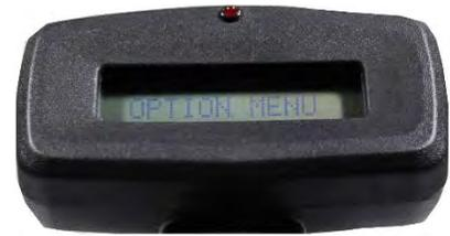
**Step 2:** The LCD will display **GO TO SURVEY?** If you want to go to survey, press and hold the Operation Button. 0 PPM will appear on the LCD. You are now ready to survey. Not pressing Operation Button will lead to next option screen.
