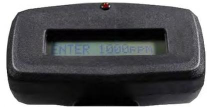
**Step 6:** Once gas and regulator are connected, press and hold Operation Button. The LCD will display **CALIBRATING** for approximately 1.5 minutes.
