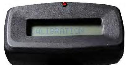
**Step 4:** The LCD will then display **ZERO CHECK** for approximately 1.5 minutes. Do not press Operation Button – wait for next prompt.
