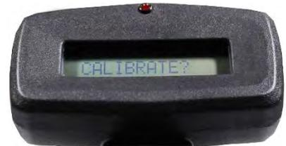
**Step 3:** The LCD will display **CALIBRATION**. Do not press button. This step takes approximately 5 seconds.
