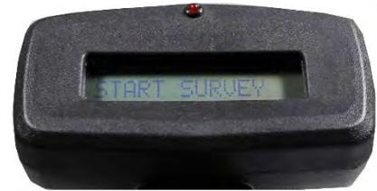
**Step 11:** If LCD displays **CALIBRATION FAIL**, check connections are secure. Check 1000 PPM calibration test gas to be correct type and above 350 psi. Next, press Operation Button for **OPTION MENU**, then choose **CALIBRATE?** and retry calibration. If **CALIBRATION FAIL** occurs again, turn unit completely off and restart in warm up mode, then try to calibrate. Call Southern Cross support if calibration fails more than 3 times at **800-241-5057**.
