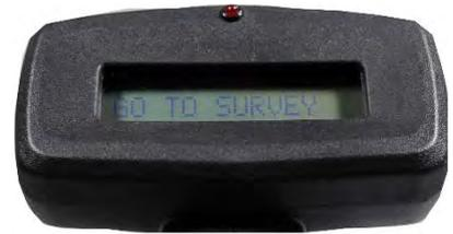
**Step 3:** Next, the LCD will display **ALARM LEVEL?** If you want to change the alarm level, press and hold the Operation Button. LCD will prompt you to choose alarm level. Press and hold the Operation Button at desired alarm level. Not pressing the Operation Button will lead to next option screen.
